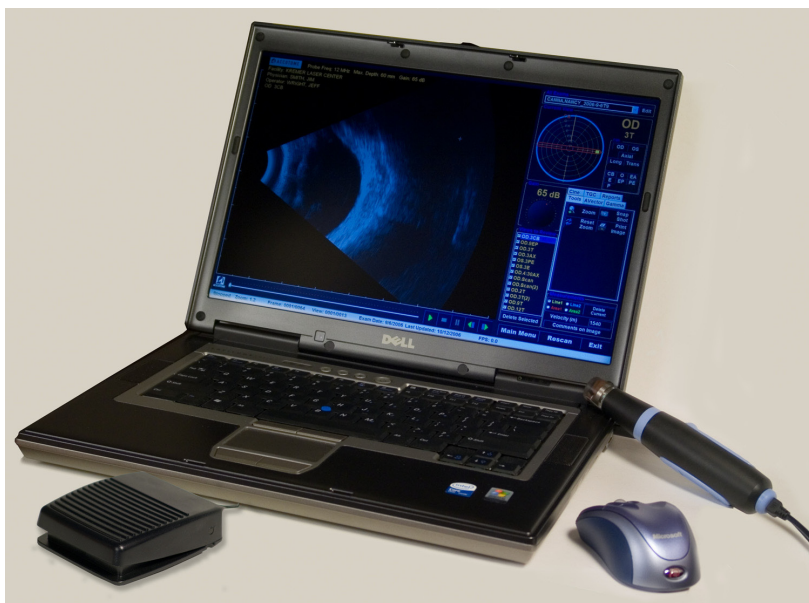
Figure 1.1 - Accutome B-Scan Plus Components
