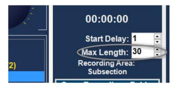
5. **Step Five:** Scan desired positions with B-Scan/ UBM probes. Video recording can be stopped by pressing F5, Stop, or once a max video length is reached. Any scanning after max length is reached will not be present in the video recording. Probe button or footswitch still needs to be pressed to stop probe from scanning.
