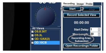
Step Six: Video recording can be opened and reviewed by using Open Recordings Folder.
