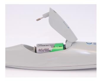
Figure 3: Battery Insertion
